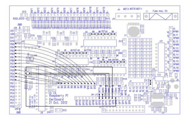
Figure 1: Gertboard wiring scheme.
